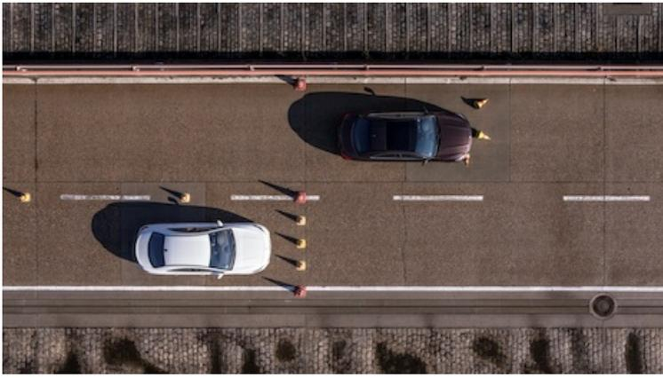
*The vehicle positioned at the top utilized phony parts, leading it to fail a brake test. Image credit: Mercedes-Benz*
